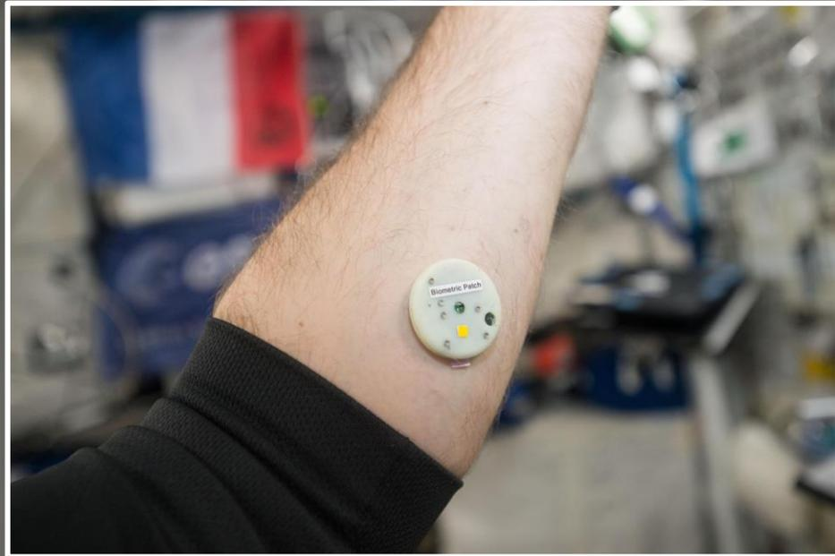
*The EveryWear assistant is an ambulatory data collection system that makes use of wearable sensors connected to a space station iPad tablet computer, which itself, is wirelessly synchronized with computers on the ground.*
